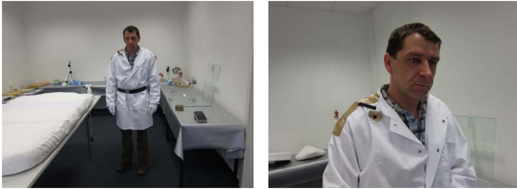
Figure 1 Positioning of the two NanoTracers and the Filter for passive sampling of airborne nanoparticles for chemical analysis by SEM/EDX. Left photo: On the table one finds the Far Field NanoTracer. Right photo: At the shoulder of the worker one finds the in-let “tube” of the NanoTracer for personal exposure measurements (the actual NanoTracer is carried at the back of the worker) and the circular “batch” for passive SEM/EDX sampling.
